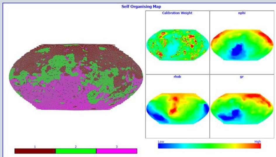
Figure 1. Example of Self Organising Maps (SOM) based on the spherical map geometry. The large map shows the SOM established from mapping of the three lithologies (shale, silt, sand) we want to predict. Maps of the three input variables used are shown also. The "Calibration Weight" map is established when calibrating the trained SOM to the facies data we want to predict. When performing this step we go from an un-supervised to a supervised SOM.
