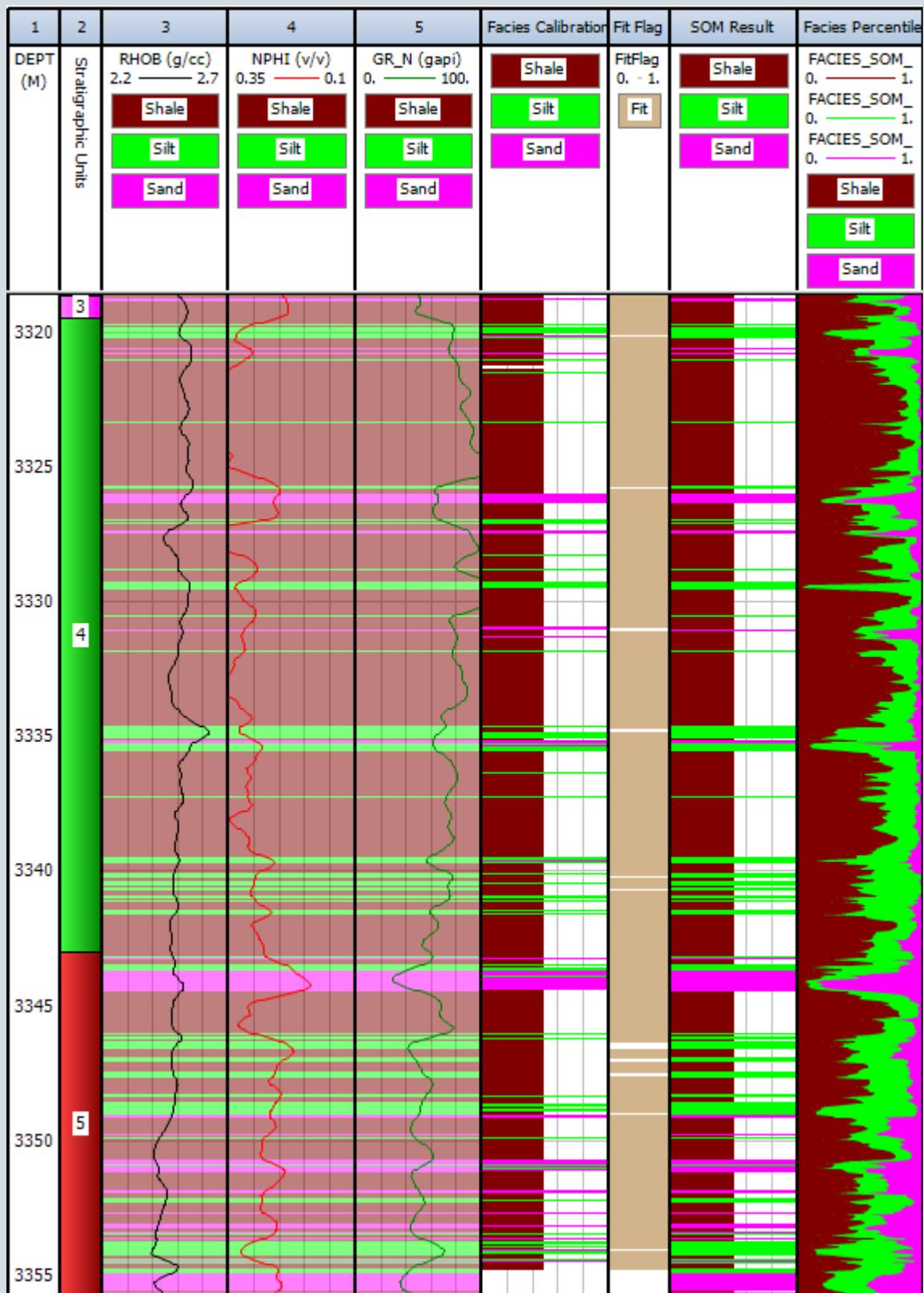
Figure 7. Well X-1 T2. The figure shows all input data as well as predicted facies from SOM over the lower part of core 1 covering mainly non-reservoir shale formations. Further explanation of the plot is found under figure 6.
