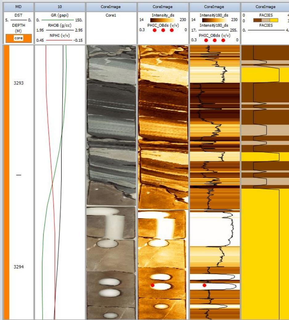
Figure 3. The core image, the intensity images and the final discrete facies log used in SOM. The three LWD log curves used as input to SOM evaluation are also shown and the challenge in terms of log resolution can be seen.
