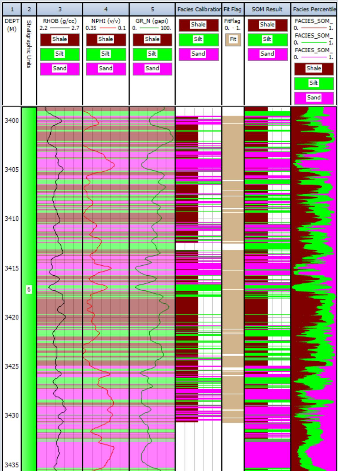
Figure 8. Well X-1 T2. The figure shows all input data as well as predicted facies from SOM over core 2 covering the major part of the deeper sand. Further explanation of the plot is found under figure 6.
