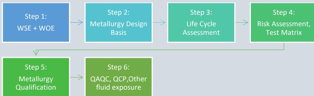
Figure 1: Metallurgy Selection Process
