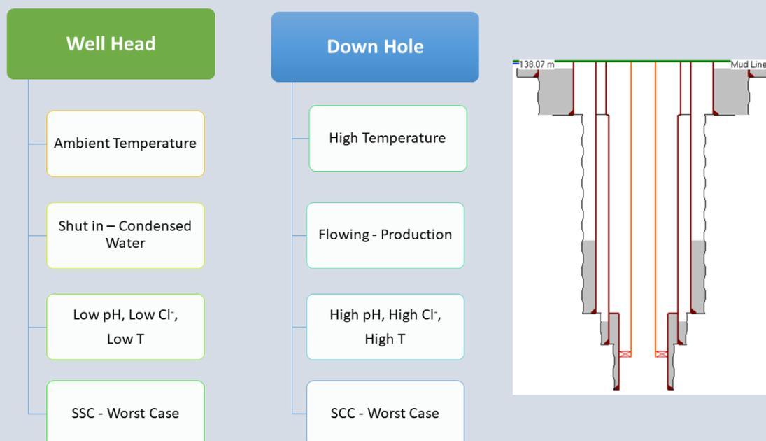
Figure 3: Worst Case illustration of SSC and SCC
